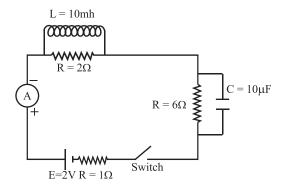
Calculate the current just (i) when switched on (ii) long time after the switching on and (iii) when turned off.
